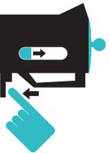
To help save wasted energy from over-filling electric kettles, a new design encourages the user to only boil exactly what they need by having two different filling chambers. One that holds the water in reserve and the other that actually boils it. A button has to be held down to fill the boiling chamber from the reserved water. This saves energy as only what is needed is actually boiled.
